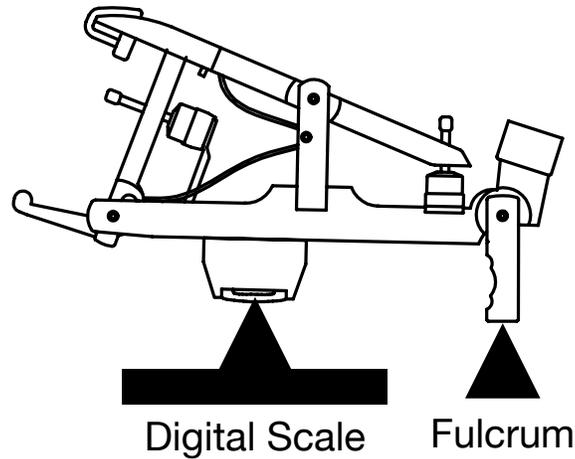
The RW is the weight at the heel/capstan contact point as read on the scale with the flange pin centred on the fulcrum or any other Friction-Free reference point.
