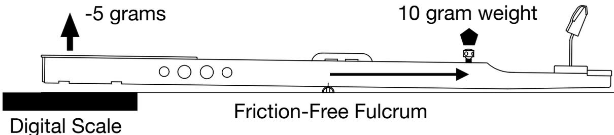
The KR is the ratio of the key front to the balance pin (fulcrum) divided by the capstan to the balance pin (as indicated by the arrow).
