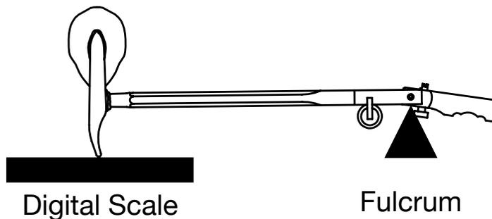
The SR is the combined hammer & shank weight as read on the digital scale with the flange pin centred on the fulcrum or any other Friction-Free reference point.
